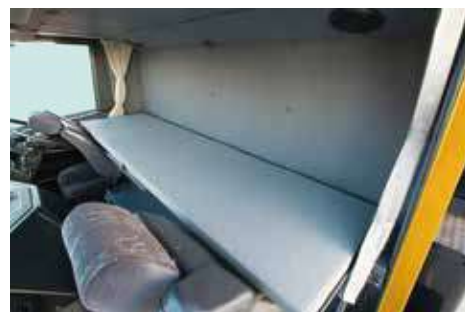
▲ large size retractable bed (2320mm×600mm)
