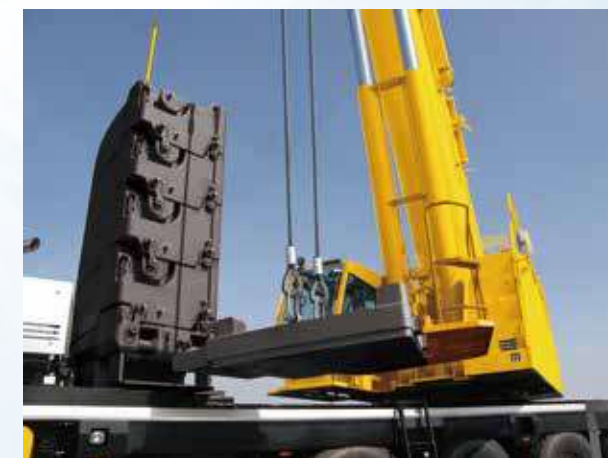
▲ Example of counterweight assembly (detaching side base)
